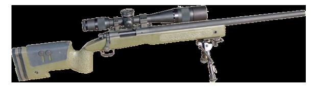
The M40A3 is a 7.62mm sniper rifle with a maximum effective range of 1000 meters. It has a 10x scope and a five round magazine.
