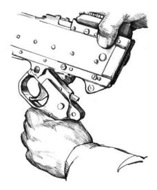
**Step 8** Disengage the holding notch at the front of the assembly from its recess on the bottom of the receiver.
