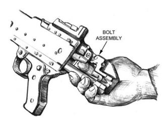
**Step 5** Grasp the bolt and operating rod assembly and remove them from the rear of the receiver.
