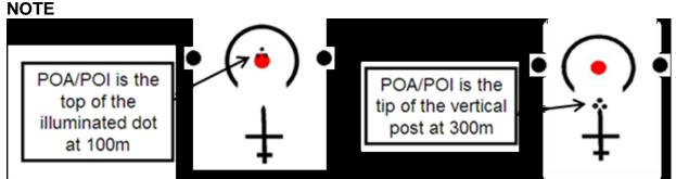
Ideally confirm 300m Zero from 300m (vertical tip is a more precise aiming point). BDC can be aligned from any known distance using the appropriate aiming point for target range.
