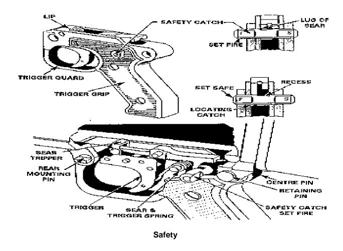
Push the safety from right to left ("F" visible) to render the weapon ready to fire. When the safety is *not* engaged, the cutaway portion of the safety bar is aligned with the safety lug on the sear. The sear is allowed to move downward when the trigger is pulled.
