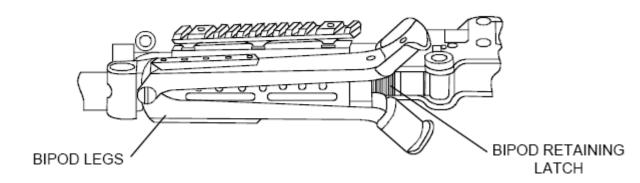
To raise the bipod legs, squeeze them together (see diagram below) and rotate the legs rearward and upward into the slot on the bottom of the receiver until the bipod latch engages, locking them in position.
