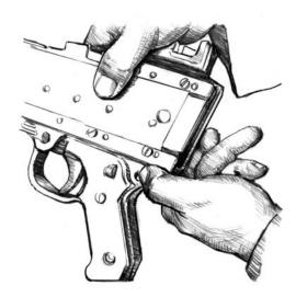
**Step 7** Rotate the rear of the trigger housing assembly down (see diagram below).
