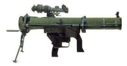
**Description.** The MK153 SMAW is a one-man, or team operable, 83 mm smooth bore, shoulder-fired, rocket launcher with a spotting rifle attached to the right side of the launcher tube. The encased rocket is fitted into the aft end of the launcher, and the fiberglass encasement is discarded after use. The spotting rifle, which improves first-round hit probability, is fed 9 mm tracers by a magazine, which holds six rounds. The 9 mm round is ballistically matched to the 83mm rocket.
