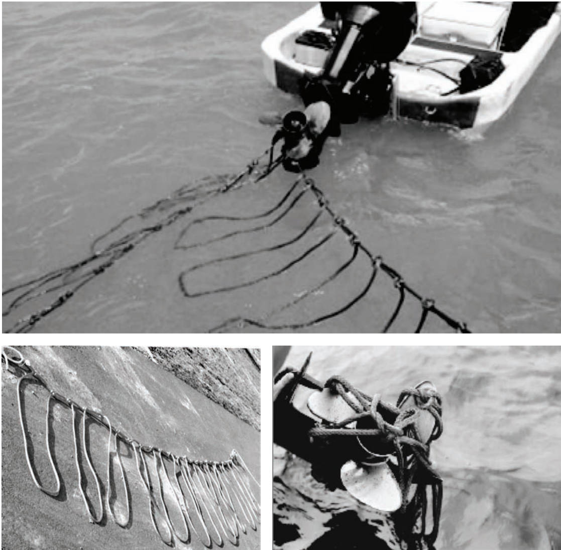
Figure D-2. Running Gear Entanglement System (RGES)
