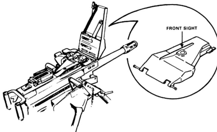
The MK19 has a leaf-type rear sight (with an adjustable range plate) (see diagram below) mounted on a spring dovetail base, which should be folded forward to a horizontal position when the weapon is moved, and which has, on the sight leaf, a range plate incremented in 100-meter intervals from 300 to 1500 meters. Range changes may be made using either the slide release or the elevation wheel:
