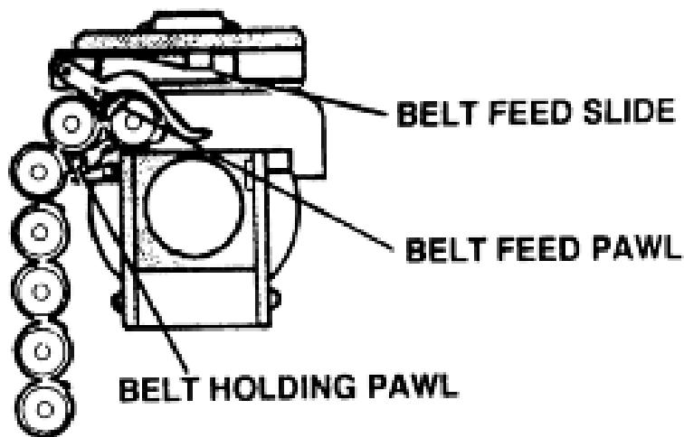
As the bolt moves forward, the belt-feed slide is moved back into the receiver, pulling with it the next linked cartridge. When the bolt reaches the fully forward position, the belt-holding pawl will snap into place behind the second linked cartridge (see diagram below), holding it in place.
