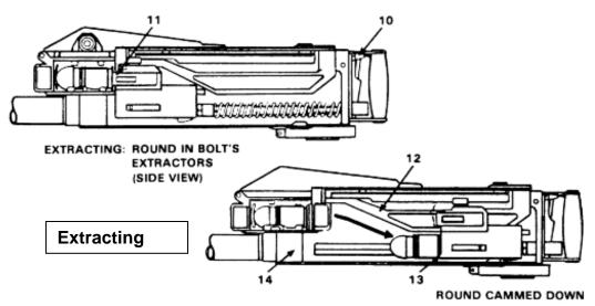
• **Ejecting:** The vertical cam forces a new round into position on the face of the bolt and ejects the spent casing out through the ejection port.
