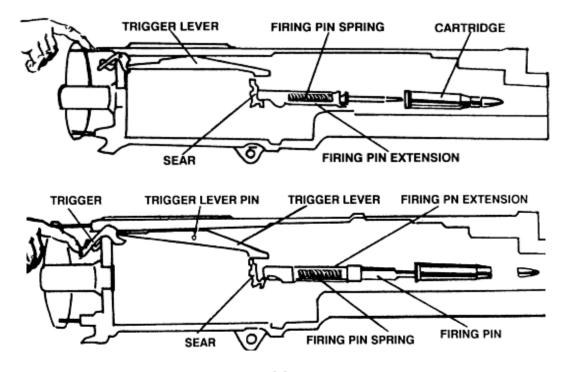
Firing M2 .50 Caliber Machine Gun Cycle of Operations (Continued)
