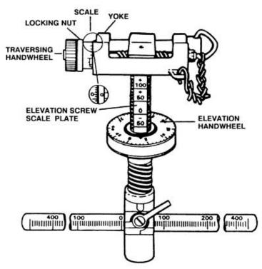
**Traversing and Elevating (T&E) Mechanism**
