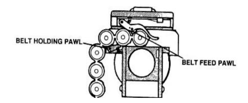
The extractor will then grasp the rim of the first cartridge, preparing to release it from the belt on the next rearward motion (see diagram below).
