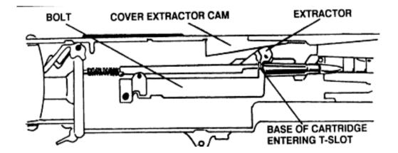
• **Chambering:** (See diagram below.) During this cycle, the bolt moves forward, carrying the cartridge in the T-slot in a direct route to the chamber of the weapon. At the same time, the extractor rides up the extractor cam and when the bolt is fully forward, the extractor grasps the next linked cartridge.
