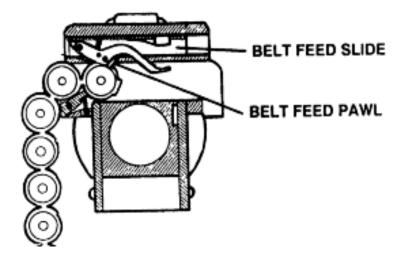
As the bolt is moved to the rear, the belt-holding pawl moves the belted ammunition over and then holds it in a stationary position. At the same time, the belt-feed pawl rides up and over the link, holding the first round in place. When the bolt is all the way to the rear, the belt-feed slide moves out far enough to allow the belt-feed pawl spring to force the pawl up between the first and second rounds (see diagram below).
