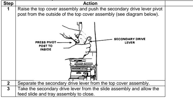
• **Removing the Top Cover Assembly**: The table below lists the steps to remove the top cover assembly.
