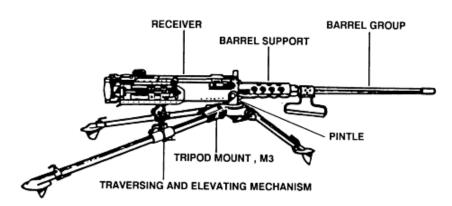
The Browning machine gun caliber .50 HB, M2 (see picture below) is a belt-fed, recoiloperated, air-cooled, crew-served machine gun. The gun is capable of single shot, as well as automatic fire, and operates on the short recoil principle. More information on the M2 will be presented in B3M4238 Heavy Machine Guns.
