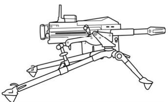
The MK19 is a belt-fed, air-cooled, blowback-operated, crew-served, fully automatic 40 mm grenade launcher. More information on the MK 19 will be presented in B3M4238 Heavy Machine Guns.
