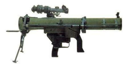
**Description.** The MK153 SMAW is a one-man operable, 83 mm smooth bore, shoulder-fired, rocket launcher with a spotting rifle attached to the right side of the launcher tube. The encased rocket is fitted into the aft end of the launcher, and the fiberglass encasement is discarded after use. The spotting rifle, which improves first-round hit probability, is fed 9 mm tracers by a magazine, which holds six rounds. The 9 mm round is ballistically matched to the 83mm rocket.
