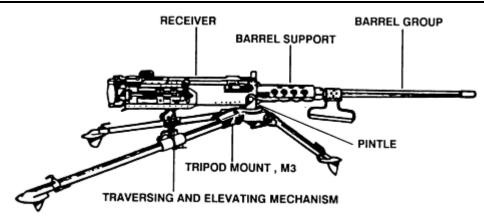
The Browning machine gun caliber .50 HB, M2A1 (see picture below) is a belt-fed, recoil-operated, air-cooled, crew-served machine gun. The gun is capable of single shot, as well as automatic fire, and operates on the short recoil principle. More information on the M2A1 will be presented in B3M4238 Heavy Machine Guns.
