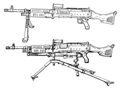
**Description.** The M240B machine gun is an belt-fed, air-cooled, gas-operated, fully automatic machine gun that fires from the open bolt position. The M240B machine gun is found in the machine gun section of the weapons platoon of every rifle company in the Marine Corps. Six of these machine guns are in each section, divided into three, two-gun squads.
