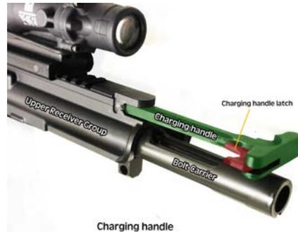
**Figure 8. Removing the bolt carrier**
