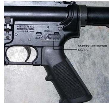
Figure 6. Selector Switch on Safe
