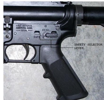
Figure 6. Selector Switch on Safe
