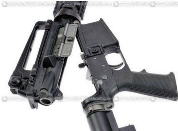
Figure 7. Detach upper and lower receiver
