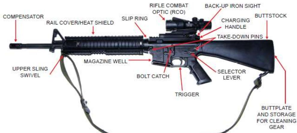
(7) The Modular Weapon System (MWS) rail enables mounting of various enhancements. The hand guards are vented to permit air to circulate around the barrel for cooling purposes and to protect the gas tube.
