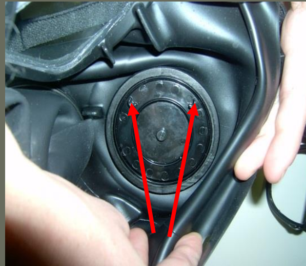
Filter mount clamp ring alignment post
